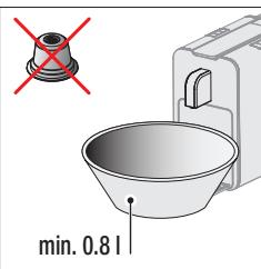
Remove all capsules from the machine, close the lever and place a **large bowl** (min. 0.8 l) under the output. If slowly lights up in light/dark, press any key
