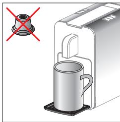
Place a cup under the output. Do not insert a capsule. If the cleaning key starts flickering slowly light/dark, press any key
