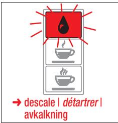
After 40 litres of coffee or tea servings the cleaning key **flashes red** during output . **Immediately** descale the machine!
